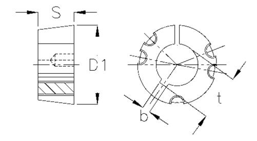
$\begin{array}{lll} b & = 14 \\ Bore & = 50 \\ Bush type & = 3525 \\ D1 & = 127 \\ S & = 64,9 \\ Screw size & = 1/2 x 1 1/2" \\ t & = 53.8 \end{array}$
